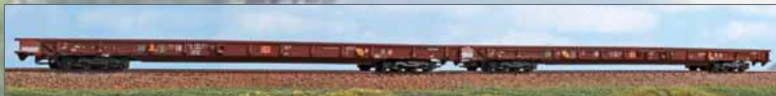
Set Rollende Landstraße DB-AG composto da due carri Tipo Saadkms per trasporto di camion. Rollende Landstraße DB-AG set composed by two Type Saadkms wagons for truck transport. Rollende Landstraße Set DB-AG bestehend aus zwei Typ Saadkms-Wagen für den LKW-Transport.
