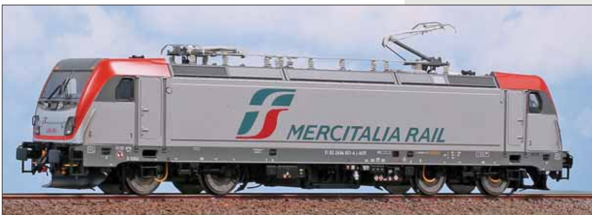
Locomotiva TRAXX 494 601 con modulo Last Mile, in livrea Mercitalia Rail. TRAXX locomotive 494 601, with Last Mile module, in "Mercitalia Rail" livery. TRAXX-Lokomotive 494 601, mit Last Mile-Modul, in „Mercitalia Rail“-Lackierung.
