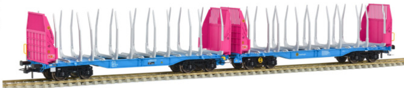
S657323 Innofreight articulated double timber transport wagon Sggmrrs | Innofreight Doppel Holztransportwagen Sggmrrs - A-IF 35 81 4657 323-5
