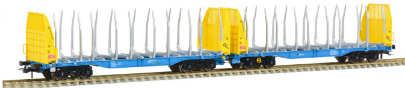
S657001 CD Cargo articulated double timber transport wagon Sggmrrs | CD Cargo Doppel Holztransportwagen Sggmrrs - A-IF 35 81 4657 001-5
